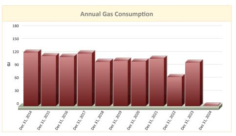
Annual gas consumption is very low for the South annex because all of the radiant floor heating and ventilation heat is generated by electrical energy, using air-source heat pumps and heat reclaim from exhaust air.
