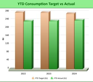
The Reliable Controls BAS calculates a daily energy consumption target in gigajoules (GJ), based on 50% of the ASHRAE standard 90.1 (1999), adjusted for actual heating and cooling degree days. Standard 90.1 is used to predict the energy consumption of an energy efficient building within a specified geographical region. Year to date for 2023, the actual energy consumed by the Reliable Controls South annex is 39.7% of ASHRAE 90.1, well below the target.
